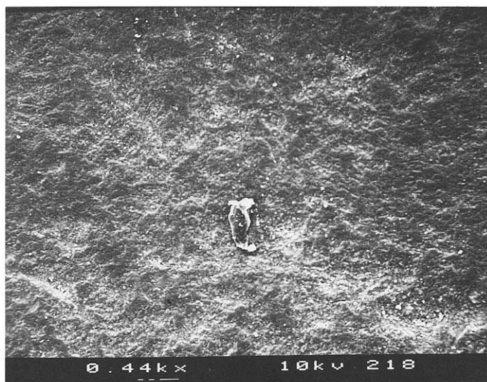
Fig. 10. SEM micrograph of the USW H-6 test well sample of the Topopah Spring Tuff at an original magnification of 44 \times .
