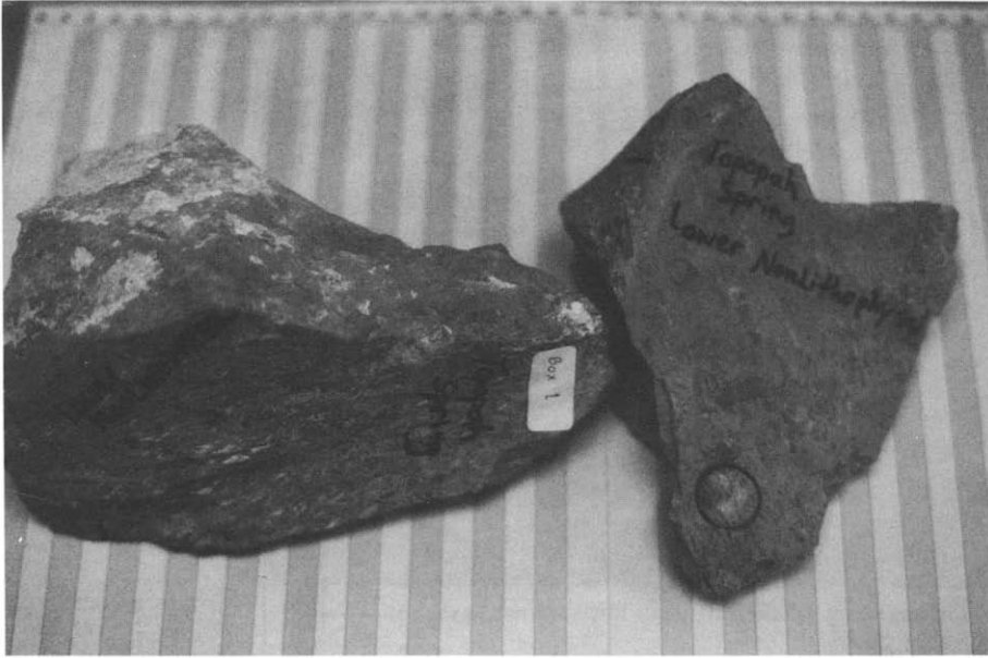
Fig. 4. Rock sample from the lower non-lithophysal zone of the Topopah Spring Tuff.
